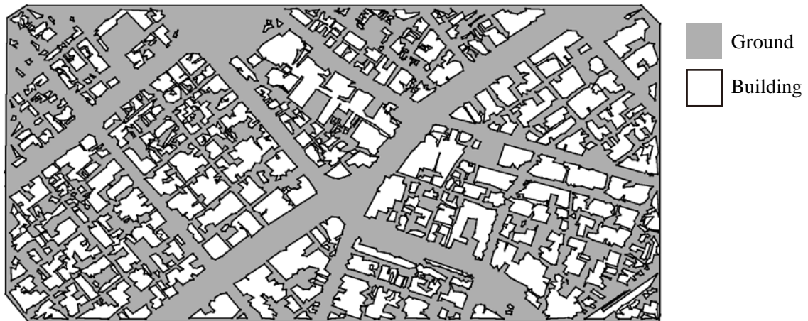
Figure 6. The flow domain boundary utilized for urban topography. The topography was obtained from an actual LiDAR survey of the city of Hyogo, Japan. In this work, a building area was treated as an impermeable wall during inundation simulations.
