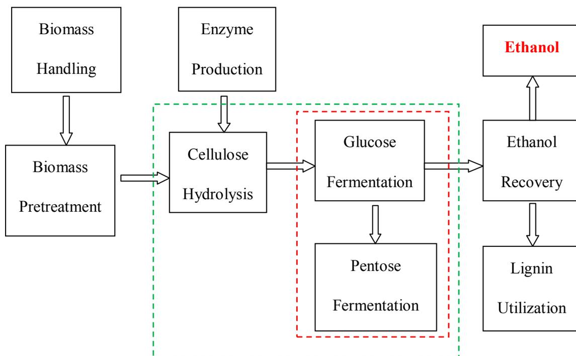
**Figure 1.2** Lignocellulosic ethanol production process (bio-chemical route).
