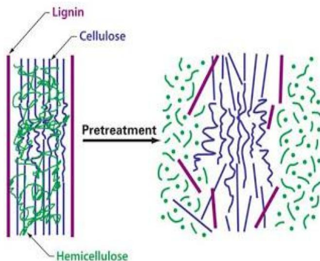
**Figure 5.1** Pretreatment of lignocellulosic biomass. (Adapted from Hsu *et al.*, 1980)
