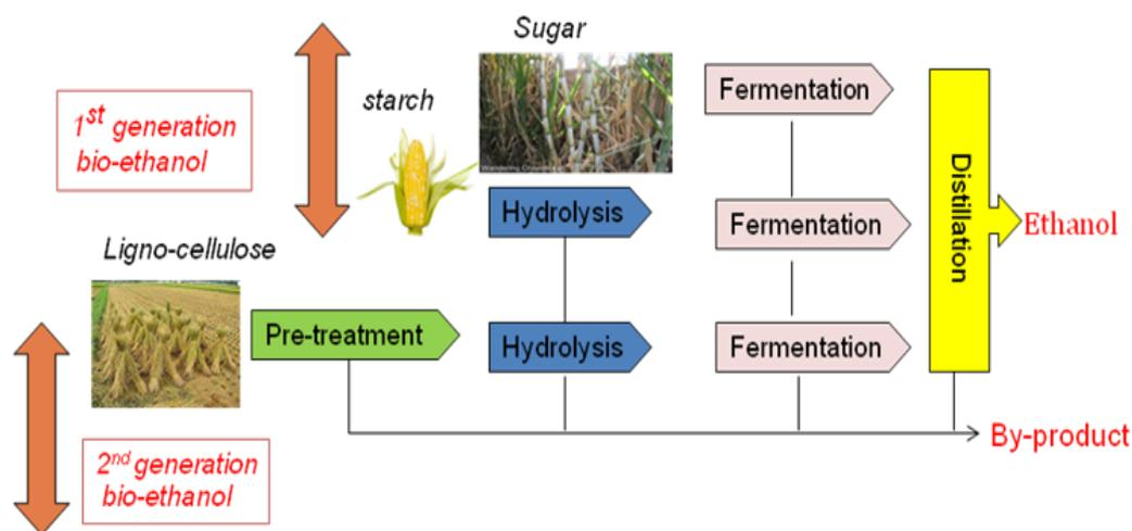
**Figure 1.1** Diagram for ethanol production from biomass.
