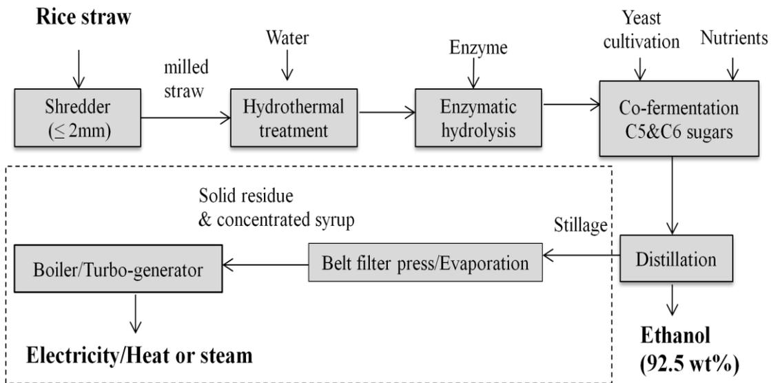
**Figure 5.2** Process flow diagram of bio-ethanol production.
