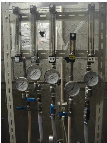
(a) Air and CH 4 rotameters with small range (AP-0250 series).
