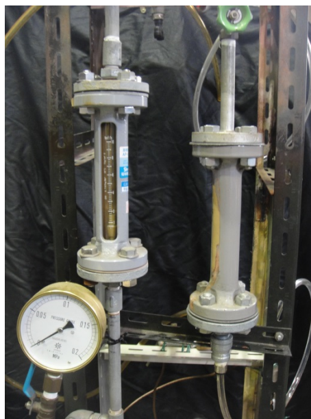
(c) CH 4 and kerosene rotameters with wide range. (left: for CH 4 , right: for kerosene, AP-0200 series)
