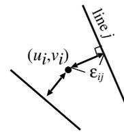
Fig. 4: Distance  $\epsilon_{ij}$  between the intersection and lines.
