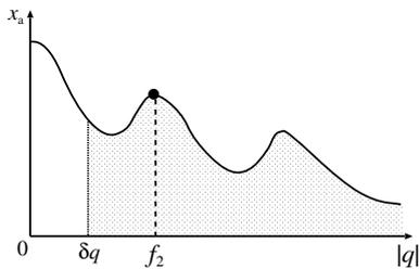
Fig. 7: Autocorrelation  $x_a$  of  $x(\mathbf{q})$ .
